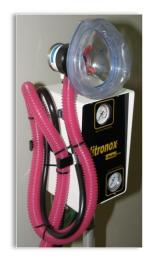
1: Firmly push one end of 19mm Corrugated Hose onto the Nitronox Scavenger.
