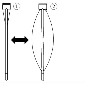
**Note:** If the reservoir bag continues to fill even after completely opening the flow control knob, check that the vacuum supply is ON, there is an adequate vacuum source pressure (10 to 21 inHg), the device is set to the correct vacuum pressure (3 to 8 inHg), the vacuum hose is properly connected, and there are no kinks in the vacuum hose. If gas continues to accumulate, contact your authorized representative for troubleshooting.
