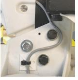
2. Locate the 3 bolts that attach the arm to the chair and remove the bolt closest to the rear of the chair. Keep the existing split washer and flat washer. Replace with 2" bolt provided placing the existing split washer and flat washer on the bolt and thread through the chair.
