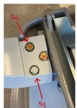
1. Remove seat upholstery to locate the 3 screws that connect the chair arm to the chair frame. Remove the bolt closest to the front of the chair for S5 Series. Remove bolt closest to the back of the chair for S4 Series.
