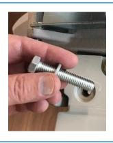
**2.** Replace existing bolt with the 2" bolt and existing split washer. Thread bolt through split washer and chair.
