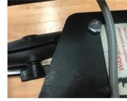
2. Thread 1" bolt through the flat washer and pre-drilled hole shown above. Underneath the mounting plate place the ball mount and lock nut on the 1" bolt. The ball mount should be orientated towards the back of the chair. Tighten with a 9/16" wrench.
