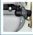
**3.** Underneath the chair arm, place the ball mount on the bolt followed by the lock nut. The ball mount should be orientated towards the back of the chair. Tighten with 9/16" wrench.
