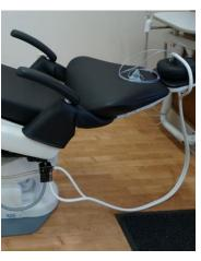
1. Remove upholstery from chair, locate the predrilled holes on the black mounting plate.
