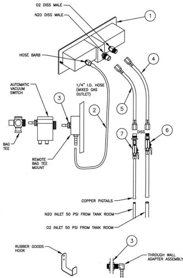
**INSTALL THE GAS LINES:** A qualified plumber can install the delivery piping up to and including the DISS Shut-Off Valves by following the details below and illustrations in this brochure.
