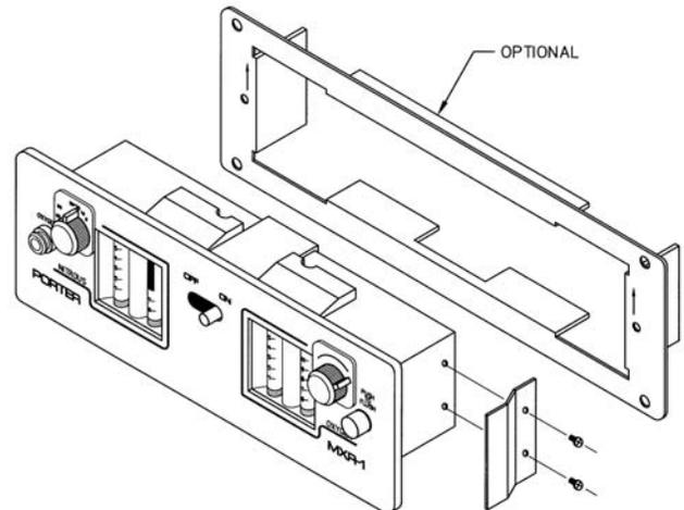
10. Pull O<sub>2</sub> and N<sub>2</sub>O DISS hoses and mixed gas hose through opening in mounting frame.
